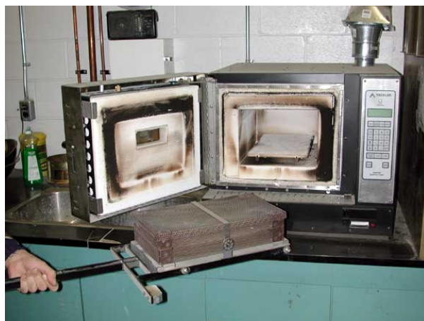
Photograph 7. The ignition oven was used for the gradation and asphalt cement testing of the mixes on the Red Hill Valley Parkway with the exception of the SMA mix.
