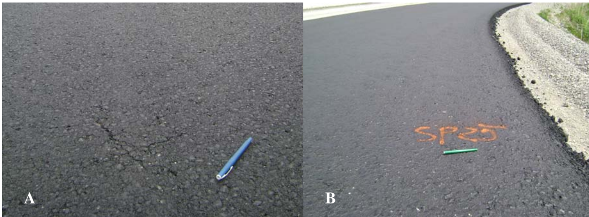
Photograph 5. Check cracking observed in the original Superpave 25 mix (A). After the mix gradation was adjusted, no check cracking was observed (B).
