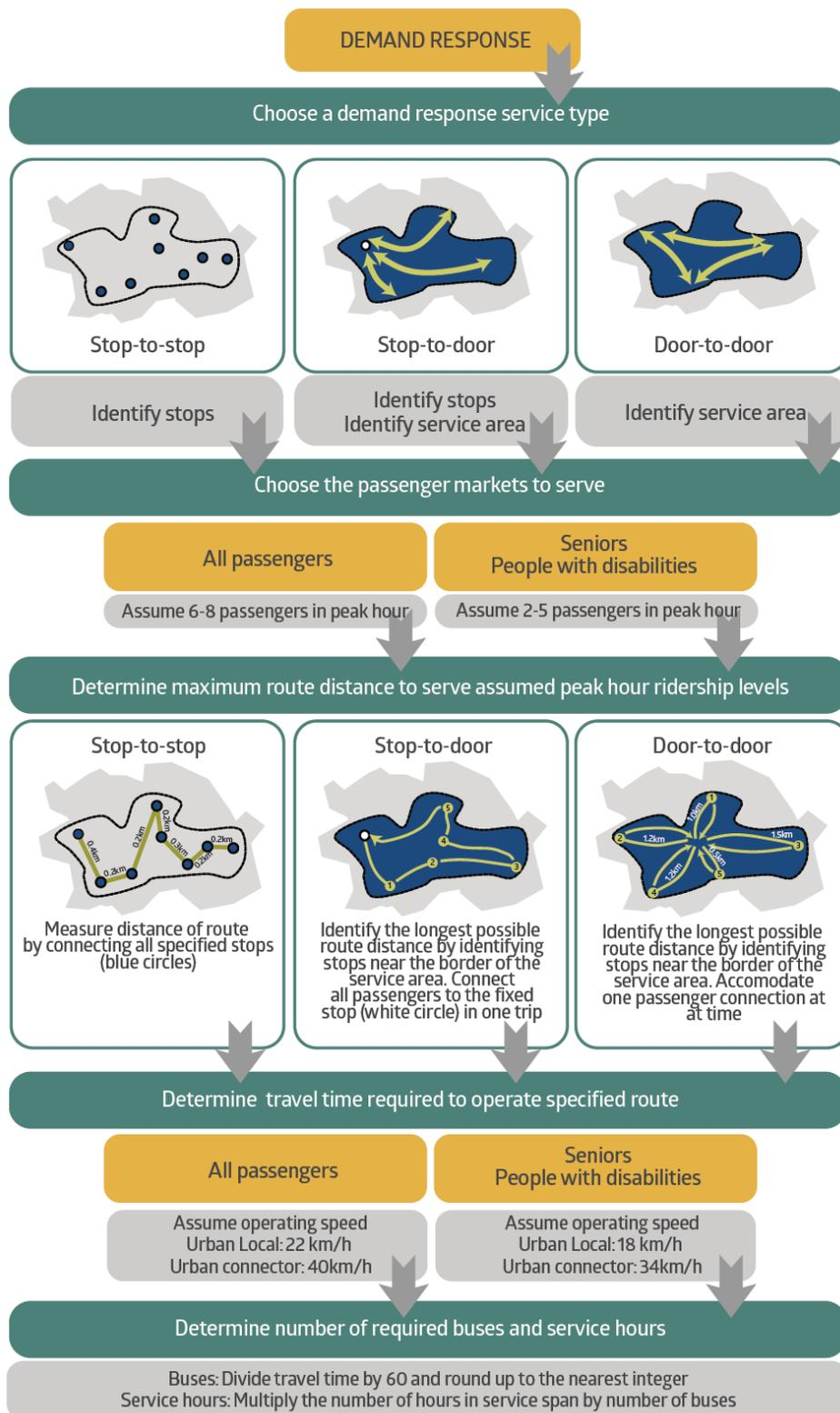
Figure 5-6 – Process for identifying demand response service characteristics
