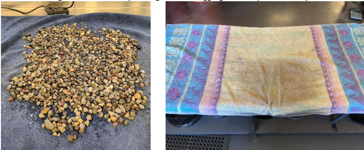
Figure 12. Laboratory Testing of Coarse Aggregates for Specific Gravity
