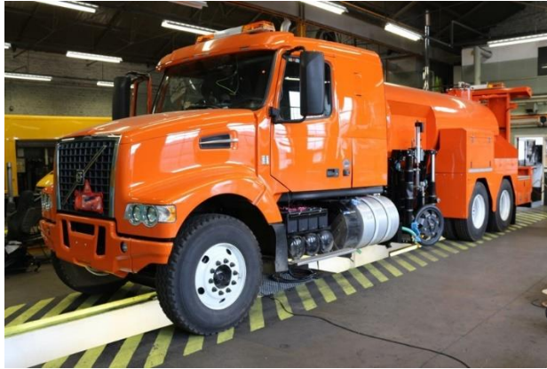
Full view of the Sideway Force Coefficient Routine Investigation Machine (SCRIM Source: FHWA)
