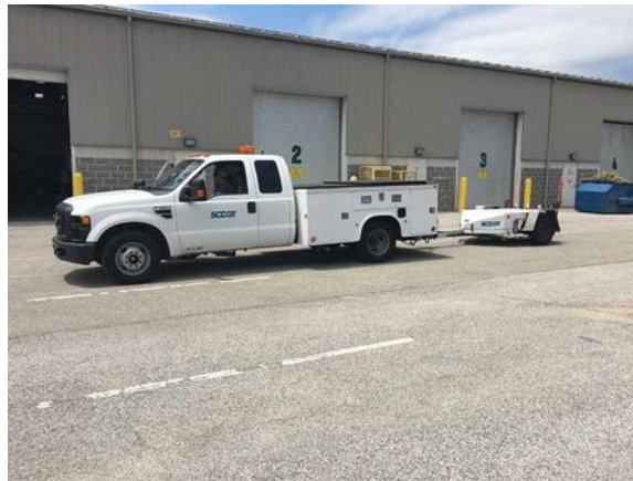
A utility truck is prepared to start an LWST owned by the South Carolina DOT. Source: FHWA
