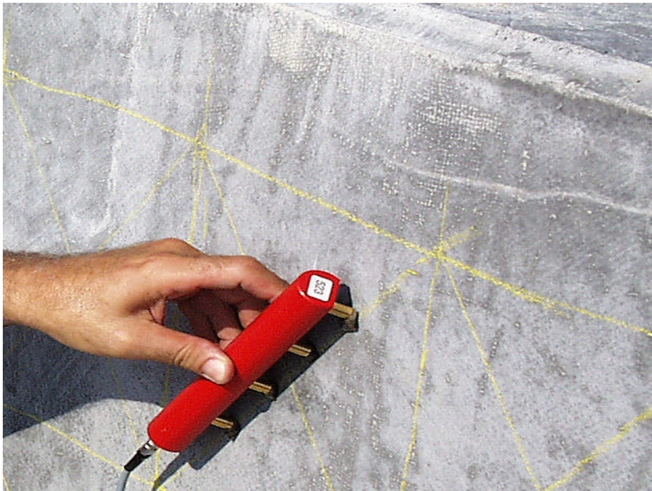
Fig. 3 Using a four-point Wenner probe to test in-situ resistivity
