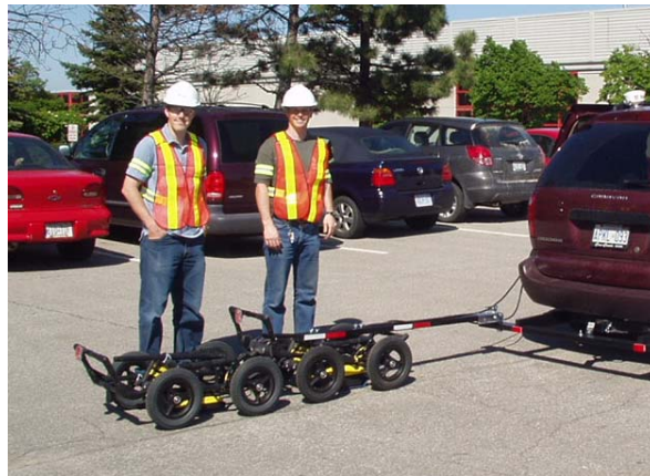
Figure 2: GPR two component system- the 500 MHz radar followed by the 1000 MHz radar
