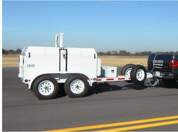
Figure 1: Falling Weight Deflectometer
